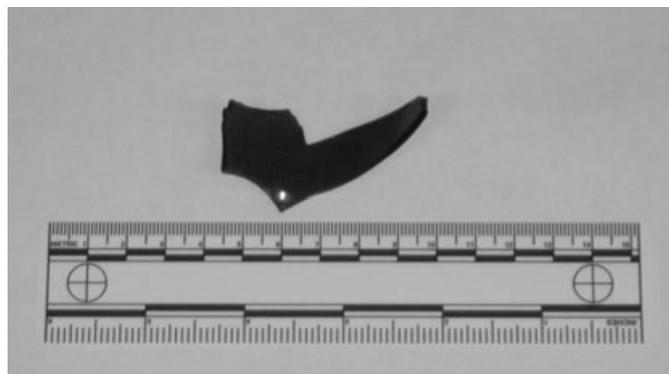
FIG. 13—Glass fragment from a bottle in which Triple Seven<sup>®</sup> was burned.
