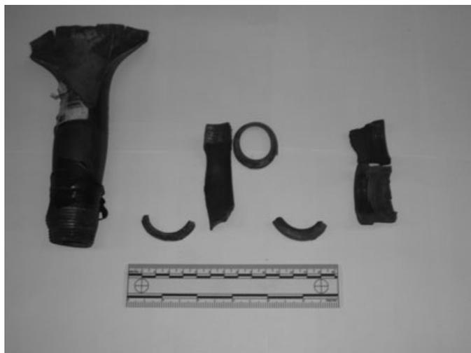
FIG. 11—Postblast debris from an 8-inch by 1-inch nominal diameter black steel pipe filled with Pyrodex<sup>®</sup> RS and initiated with an electric match. RS, Rifle/Shotgun.
