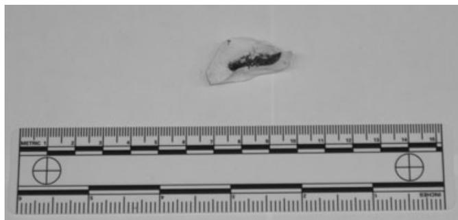
FIG. 9—Postblast fragment from a 8-inch by 1-inch nominal diameter PVC pipe filled with Pyrodex<sup>®</sup> RS and initiated with an electric match. RS, Rifle/Shotgun.
